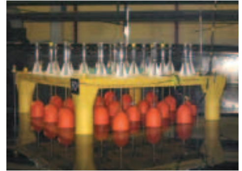
1:20 model in the wave tank with 21 point absorbers/eggs installed on a floating platform.
